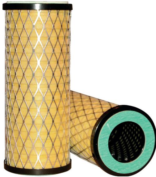
Facet's Model MG glass fiber depth filter cartridges are for removing colloidal, slimy or sludge type solids 10 micron and larger or where compatibility problems exist with cellulose media.
