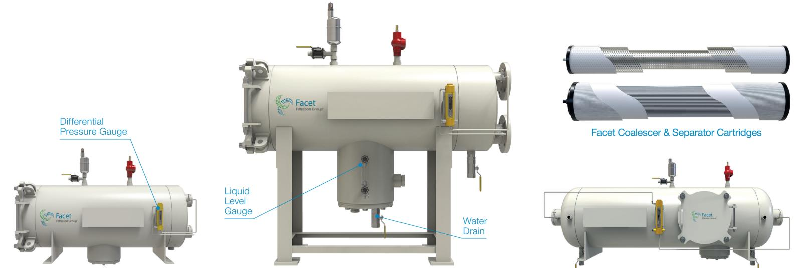
Filter water separators are the primary defense against fuel contamination by water and dirt. These housings contain both first-stage coalescer and second-stage separator cartridges with no internal moving parts to continuously remove solids and water contaminants from aviation fuels.
