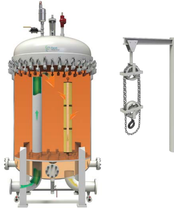
Typical Clay Treater Housing Flow Diagram (Including optional items)
