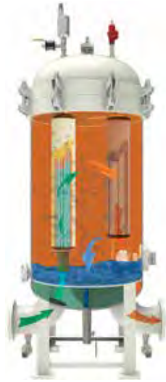
Vertical Two-Stage Coalescer Separator Flow Diagram
