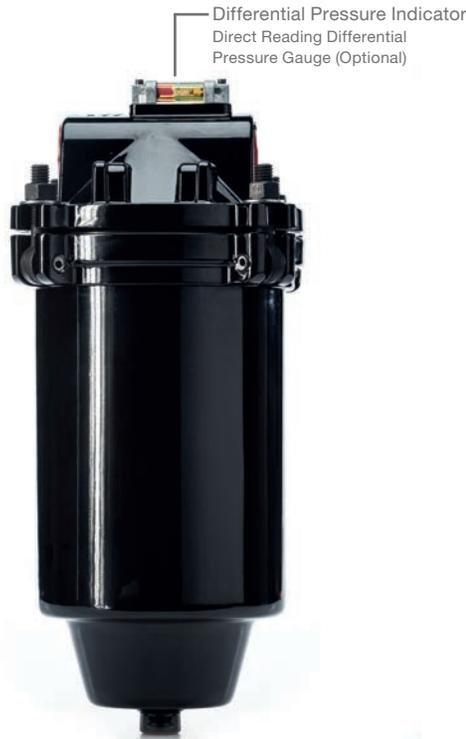
The Facet VF-21SB/22SB can be used as a filter housing. They are versatile, compact, light weight housings and provide superior in-line filtration protection. Both interior and exterior surfaces of the carbon steel body are epoxy coated to protect against corrosion. This sturdy, single cartridge housing is easy to maintain and requires only 2" (51 mm) base clearance for cartridge change out.
