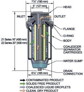
These housings installed with one Fuel-Gard® monitor cartridge, will continually check the entire flow of fuel, not just mere samples, for water or solids contamination. By performing three jobs, this small compact monitor assures clean, dry fuel. It absorbs free and emulsified water, removes ultra-fine solids, and shuts down system flow when hit with a localized slug of water. Both interior and exterior surfaces of the carbon steel body
