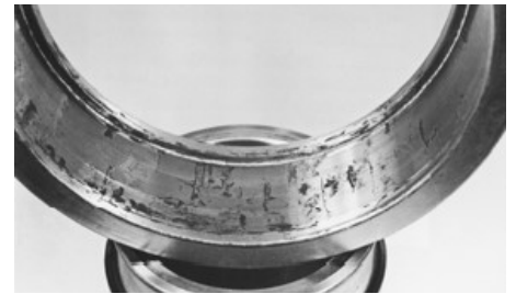
Bearing failure from excess water
