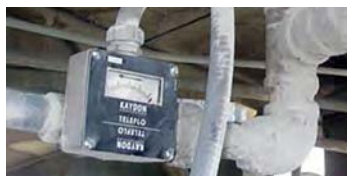
Close-up view of Model 816BC TELEFLO Flow Switch mounted on rock crusher lube oil (ISO 150) circuit for protection against loss of oil flow in quarry application.
